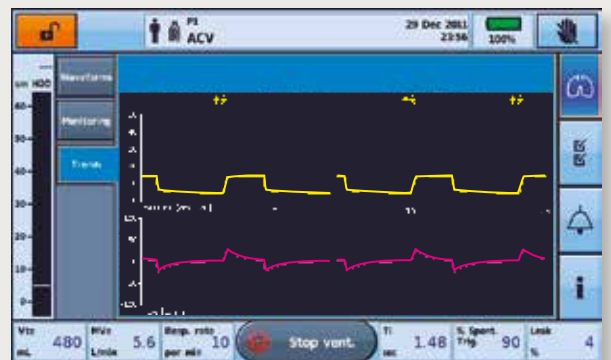
Real-time pressure and flow waveforms display essential therapy parameters on the large touchscreen.
